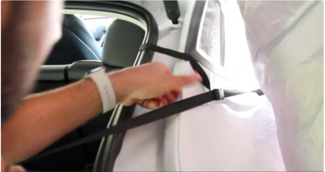
Middle two straps interconnect around rear pillar
